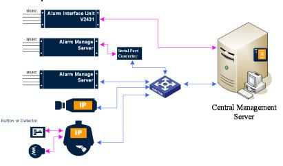
codes are managed centrally and are routed automatically to the V2216 management platform CMS module. Alarms from all edge devices are managed in a uniform way using dedicated alarm code in the software to switch video to monitors and display maps to show where the alarm originated.
