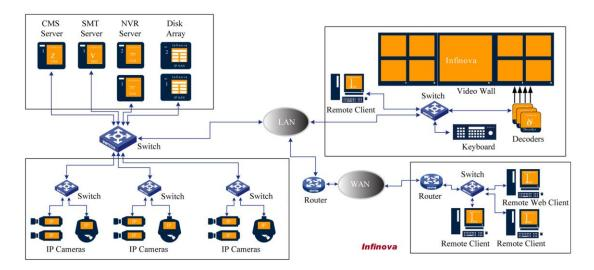
Cameras are located in all areas of the plant, for example the main dam, upper river area of the reservoir, flood discharge tunnels, flood gate control room, hydraulic turbine floor, transformer station and switch room. The cameras are all IP and are connected to the command center via local switched and a fiber optic LAN.
